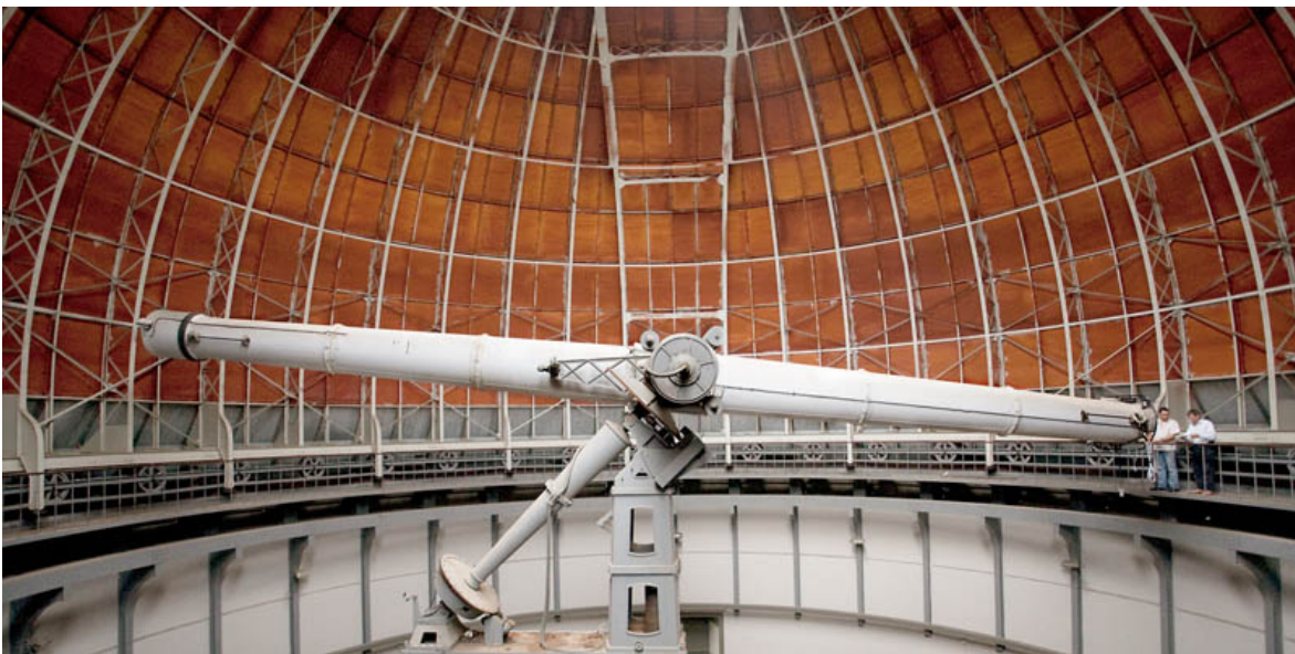
Figure 3.2: The 76cm diameter refractor's tube in the " Grand Equatorial " dome, at the Observatoire de la Côte d'Azur, on which prototype generation II will be installed.
