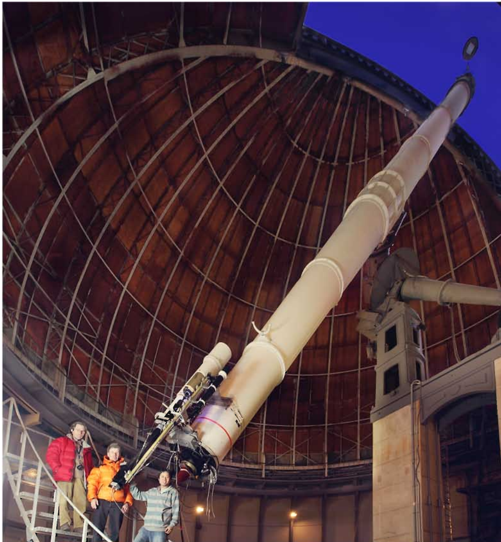
Figure 1. Fresnel generation II testbed on the side of the 18 meter refractor at Observatoire de Nice. The 20 cm square Fresnel array is attached to the front end, the receptor module is the thin steerable optical bench at the rear end. The optical axis of the Fresnel imager runs in free air outside the refractor tube.
