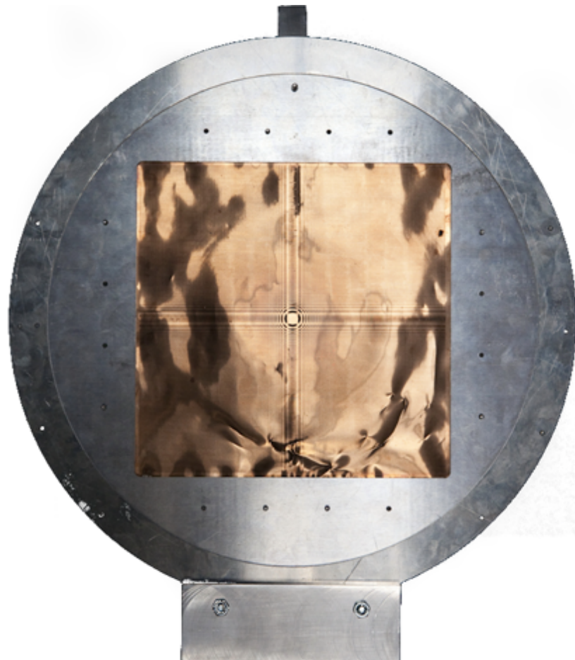
Figure 3.9: Fresnel Array in Generation II prototype, this array is 20 by 20 cm made of a thin metal foil with approximately 250000 apertures. It is held by a mechanical support allowing rotation around its optical axis in order to orient the spikes correctly in the image plane.
