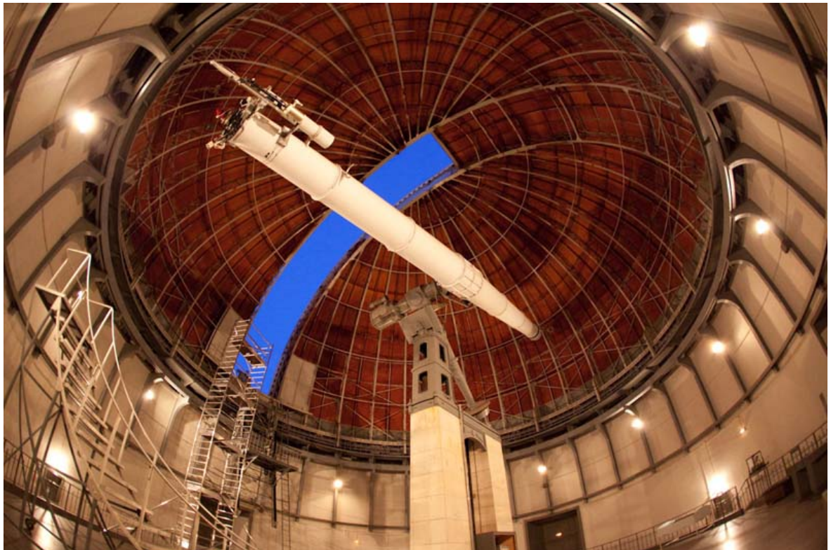
Figure 4.1: Refractor and Grand Equatorial dome at Observatoire de la Côte d'Azur: the refractor is 19 meters long and the refractor dome is 24 meters in diameter. The Fresnel array can be distinguished on the right at the far end of the tube. The receptor module on its optical rail can be seen on the left at the close end below the white finder.
