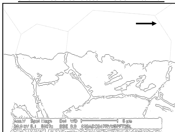
Fig 14(d). Previous austenitic grain network crack path. Edge detection on micrograph with Matlab®
