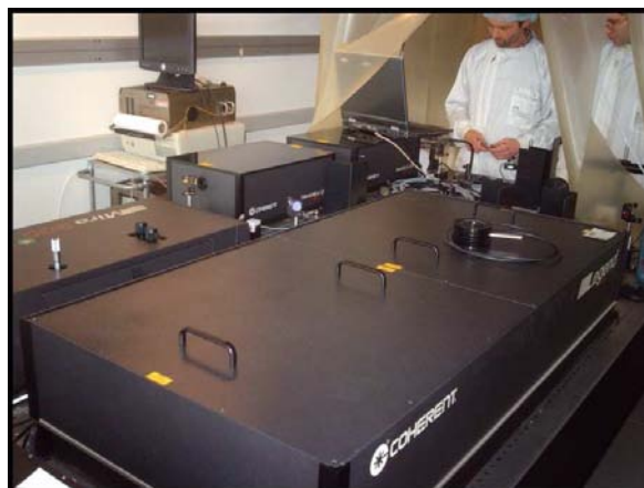
Figure II.15 : Laser Femtoseconde IR/UV de type Legend (Coherent).
