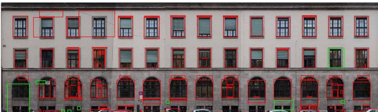
Figure 20: Replacement of small areas of connected components (red) by bounding boxes of points behind the façade (green)
