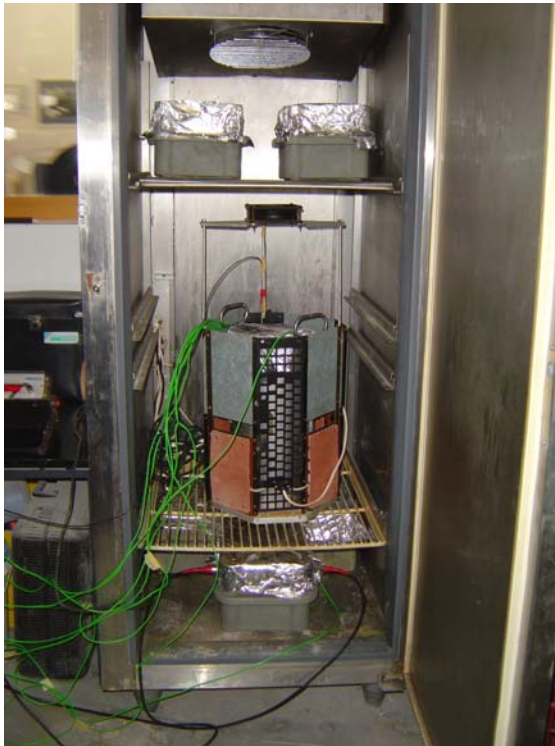
Figure 1: Adiabatic calorimeter of Building Materials Institute IGMAT
