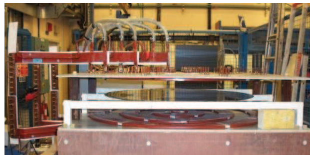
Fig. 4. Induction heating device coils, disc and bus-bar.
