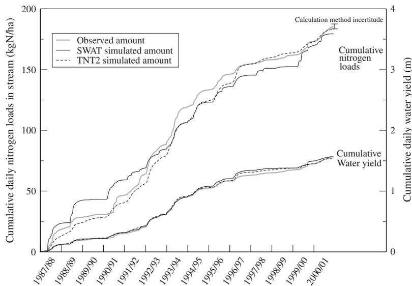
**Fig. 12.** Cumulative daily water discharge and N loads observed and simulated at the outlet of the Auradé catchment, simulated by SWAT (full line) and TNT2 (dotted line) from 01/10/1987 to 01/09/2001. Discharge are given in m and N loads in  $\text{kg N ha}^{-1}$ .
