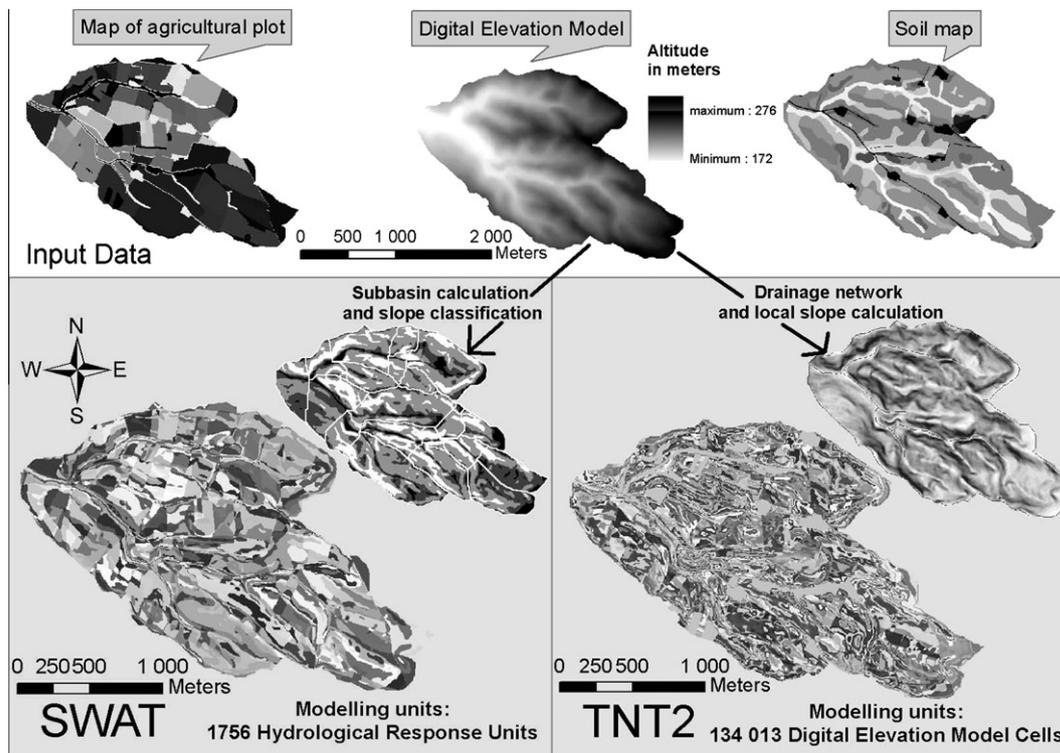
**Fig. 3.** Spatial data used in TNT2 and SWAT: soil map with 14 soil types (12 agricultural soil types, 1 for urban area and 1 for forest), DEM (5 × 5 m), agricultural plot map (92 agricultural plots). Integration of these data are detailed for fully distributed model TNT2 and semi-distributed model SWAT.
