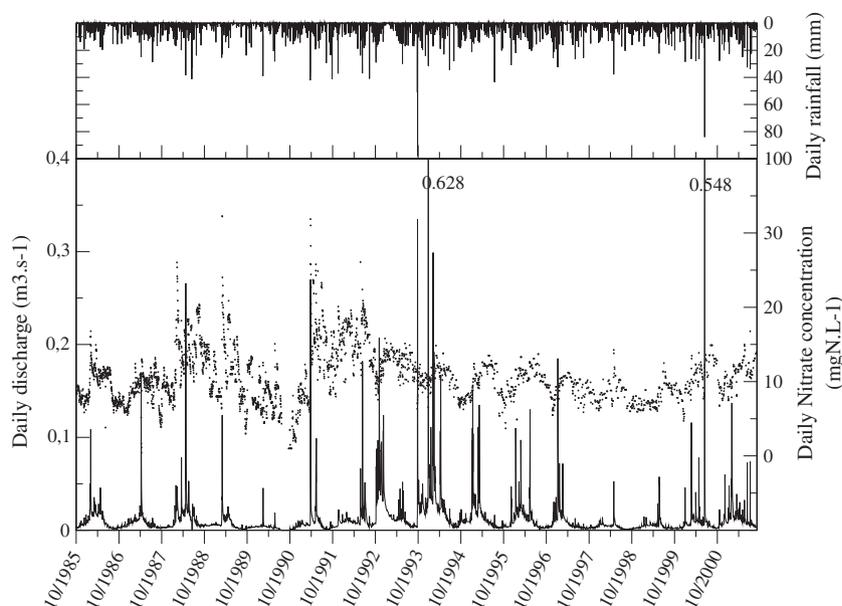
Fig. 2. Daily discharge ( $\text{m}^3 \text{s}^{-1}$ ), rainfall (mm), N concentration ( $\text{mg N-NO}_3^- \text{L}^{-1}$ ) measured in Montoussé river, at the outlet of auradé basin. source: GPN-Total.
