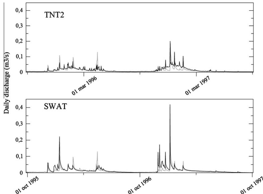
**Fig. 5.** Daily discharge (m<sup>3</sup> s<sup>-1</sup>) observed (gray line) and simulated (black line) with semi-distributed model SWAT and fully distributed model TNT2 at the outlet of Auradé from October 1995 to October 1997.
