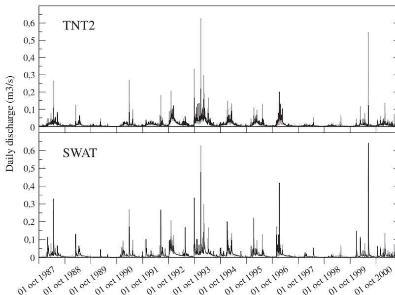
Fig. 4. Daily discharge ( $\text{m}^3 \text{ s}^{-1}$ ) observed (gray line) and simulated (black line) with semi-distributed model SWAT and fully distributed model TNT2 at the outlet of Auradé. Nash-Sutcliffe coefficient is 0.5 and 0.6 for respectively TNT2 and SWAT simulations.
