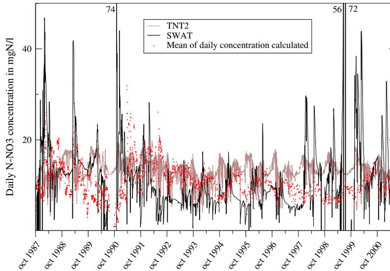
**Fig. 13.** Simulated and mean of daily concentration calculated from observed data during the study period (from October 1987 to September 2001). Mean daily concentration has been calculated from measured concentration for 2834 days of the 5814 days studied.
