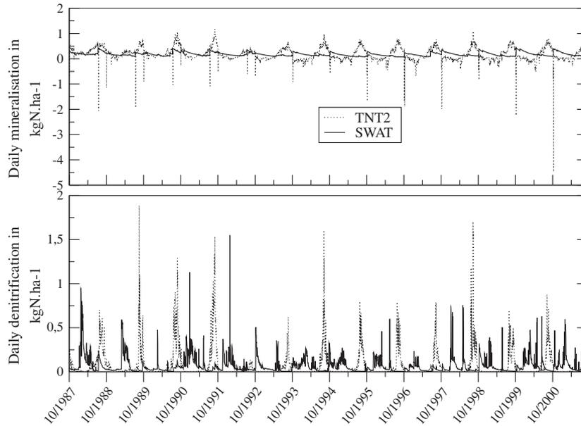
**Fig. 8.** Daily net mineralization (figure on the top) and denitrification (figure below) simulated with SWAT (gray line) and TNT2 (black line) during the study period (from 01/10/1987 to 01/09/2001). Values are given as the daily mean for the Auradé catchment in  $\text{kg N}\cdot\text{ha}^{-1}\cdot\text{day}^{-1}$ .
