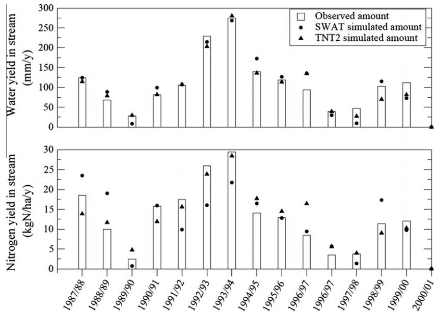
**Fig. 6.** Annual discharge and N loads (mm and kg N) observed and simulated with semi-distributed model SWAT and fully distributed model TNT2 at the outlet of Auradé from year 1987–1988 to year 2000–2001. RMSE of annual discharge are 0.018 and 0.022 mm for respectively TNT2 and SWAT. RMSE for annual load are 78.6 and 65 kg N for respectively TNT2 and SWAT.
