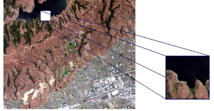
Fig. 11. Real hyperspectral data: Moffett field acquired by AVIRIS in 1997 (left) and the region of interest shown in true colors (right).
