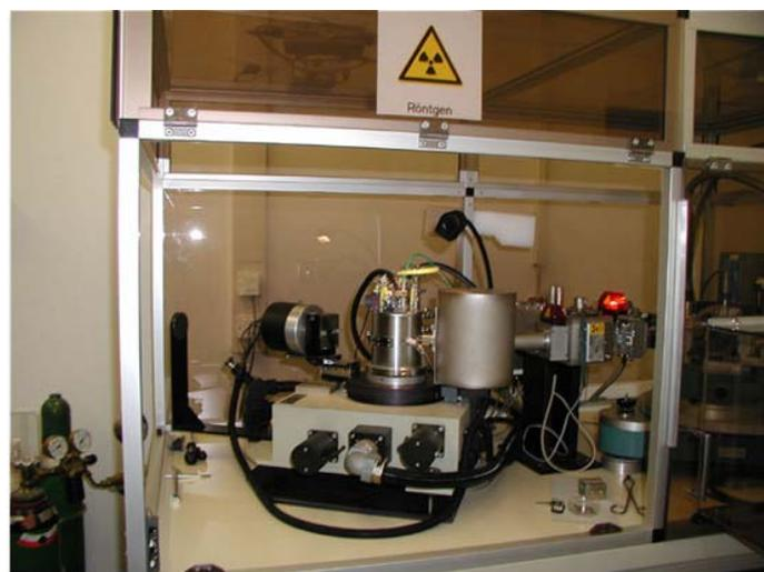
**Abb.4:** Pulverdiffraktometer [87]
