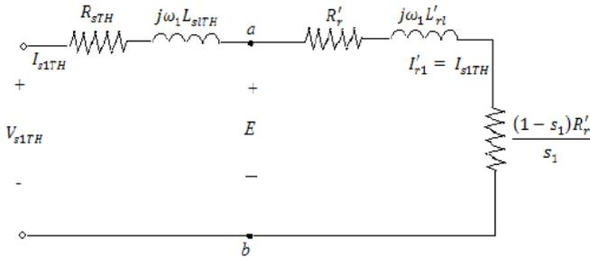
Fig. 2. Thevenin adjusted Equivalent Circuit of Three-Phase Induction Motor
