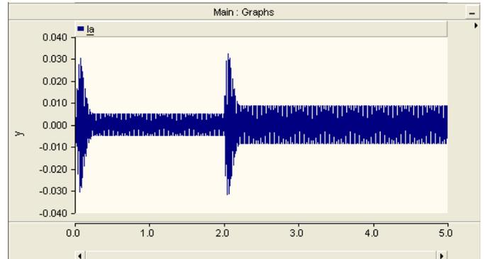
Fig. 13. Two times of Inrush Current during the Star-Delta Starting method
