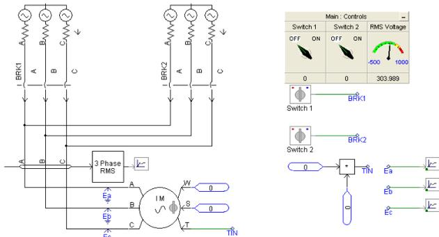
Fig. 15. Star-Delta Starting Circuit Implementation in PSCAD
