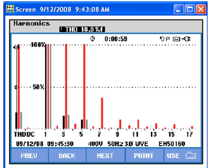
Fig. 8. Harmonics in Autotransformer Starting
