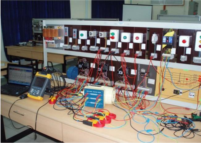
Fig. 3. Laboratory Workbench for the Motor Starting Experiment.
