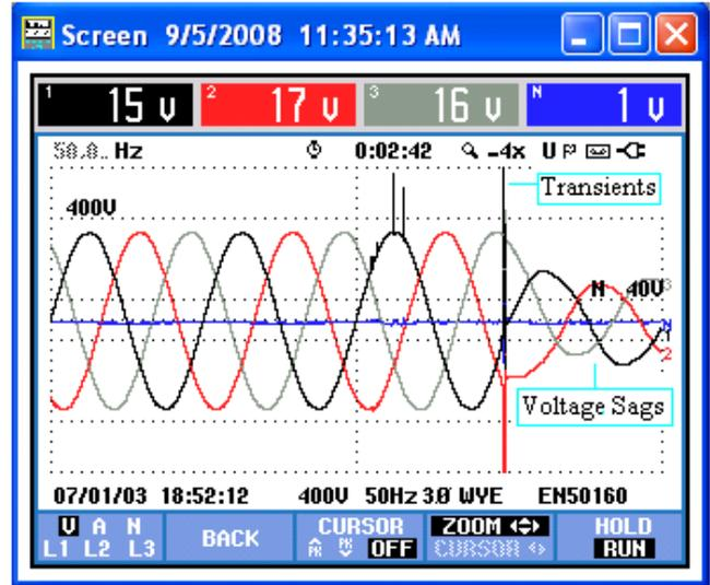
Fig. 5. Voltage Sag in DOL Starting.
