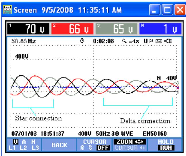
Fig. 6. Voltage Sag in Star-Delta Starting
