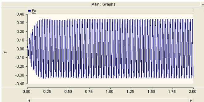
Fig. 11. Unbalanced Voltage in Direct-On-Line Starting
