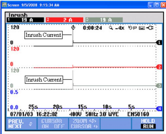
Fig. 4. Inrush Current in Direct-On-Line Starting.
