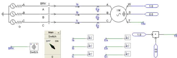
Fig. 12. Direct-On-Line Circuit Implementation by using PSCAD software
