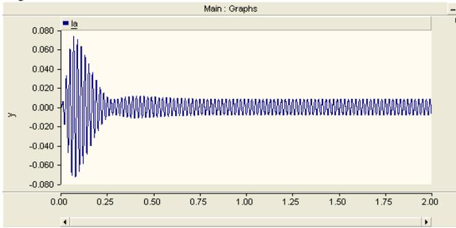
Fig. 10. The Inrush Current exists during the Direct-On-Line starting
