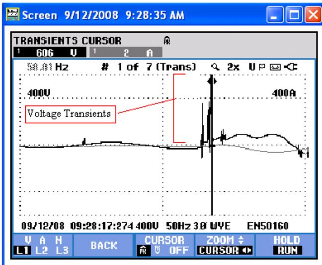
Fig. 7. Transients in Autotransformer Starting
