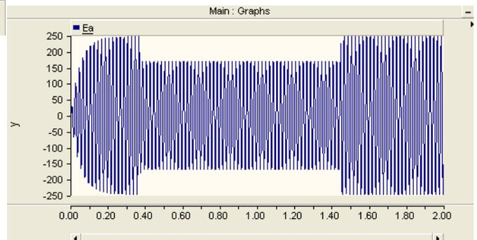
Fig. 14. Voltage Sag in the Induction Motor's Terminal A
