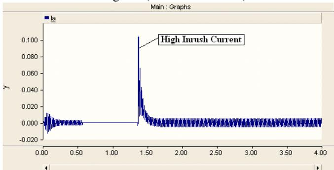
Fig. 16. Inrush Current in Autotransformer Starting
