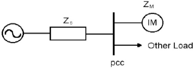
Fig. 1. Equivalent circuit for induction motor starting.
