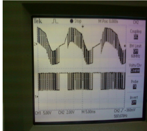
Fig.15: Voltage output of the half bridge of the H-bridge shown in channel 2 of the oscilloscope
