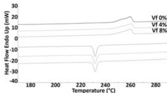
**Figure 3.** DSC thermograms of injection-moulded short glass fibre composites under dry condition (curves were shifted vertically for clarity).
