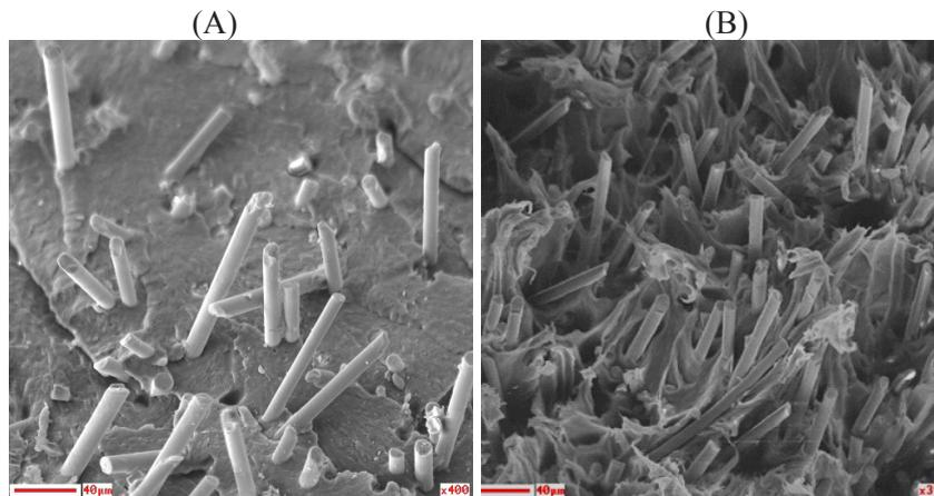
**Figure 8.** SEM micrographs of tensile fracture surface of glass fibre composites under (A) dry as-moulded and (B) wet conditions.
