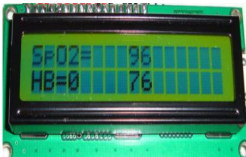
Fig 7. The Liquid Crystal Display (LCD) screen showing an example results
