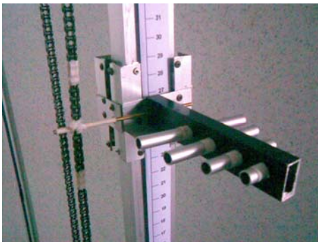
Figure 9. Testing of the accuracy of the antenna positioning device
