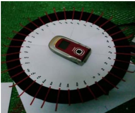
Figure 8. Testing of the accuracy of the turntable
