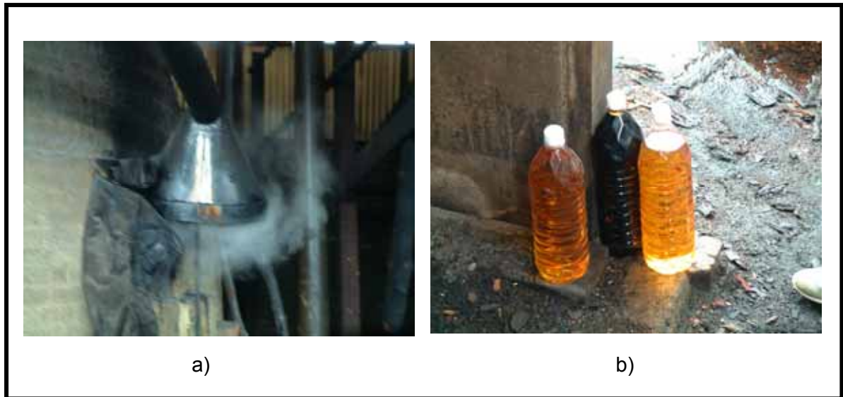
Fig. 1.6 The stainless steel pipe for collection of the condensed smoke coming out from the orifice of the charcoal kiln. The reddish brown liquid or pyroligneous acid obtained during the second stage as the result of the condensation of wood smoke (a). The product, after elimination of pyroligneous acid was a thicker, greenish black liquid (b).
