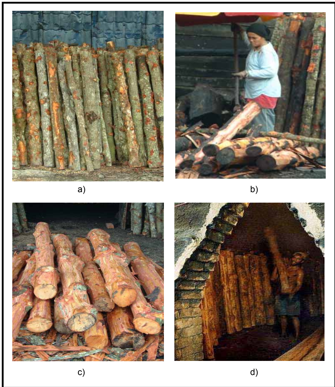
Fig. 1.4 Preparation prior to the charcoal making process at Kuala Sepetang charcoal village. The 1.6 m log of Rhizophora apiculata woods (a), the wood debarking procedure (b), the debarked woods (c) packing of the debarked woods into the charcoal kiln (d).
