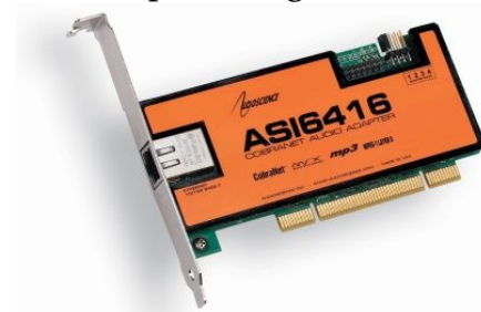
Audio card equipped with Ethernet connector
