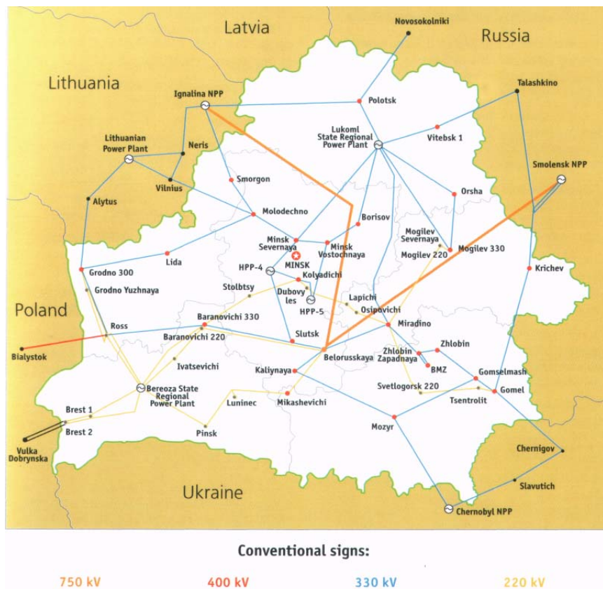
Figure 1: Power system of the Republic of Belarus
