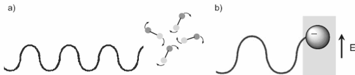
Figure-2 (a) Dipolar polarization mechanism (b) Dipolar molecular try to align with an oscillating electric field. Ionic conduction mechanism: Ions in solution will move in the electric field.
