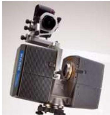
Figure 4: FARO Photon 120 integrated with Nikon DSLR 300s
