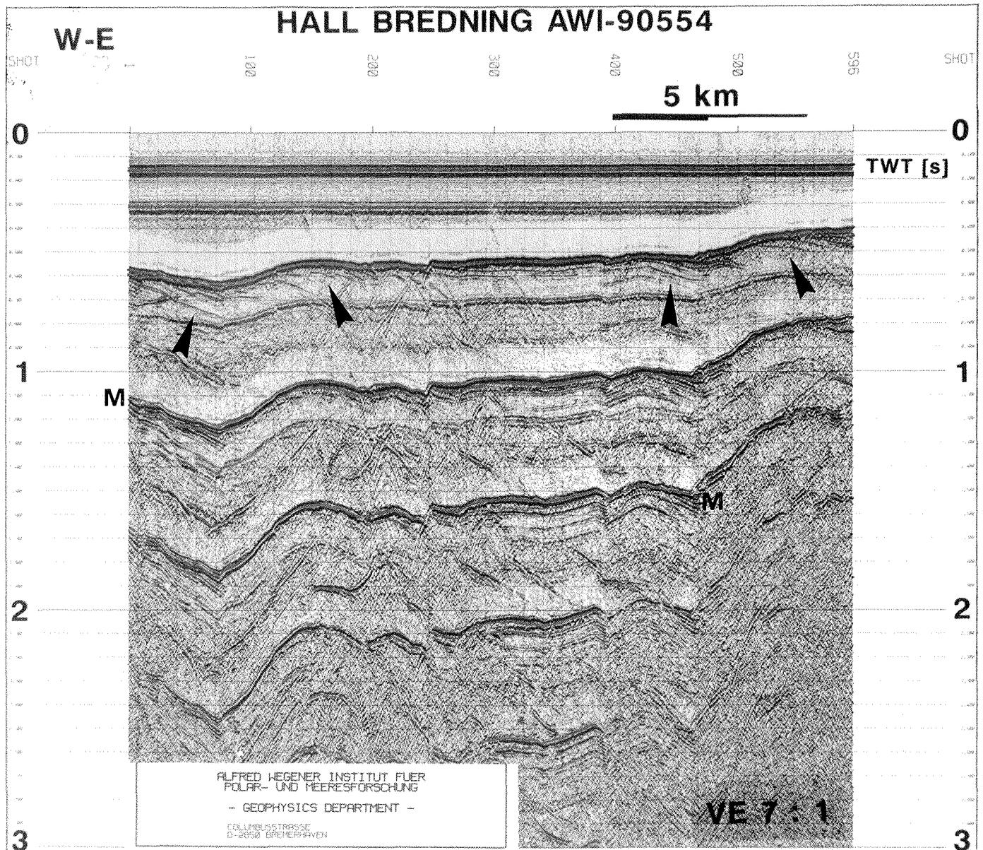
**Fig. 3:** Line AWI-90554. This profile crosses Hall Bredning from west to east. The arrows indicate dipping internal reflectors of the lower seismic sequence, whose amplitudes are small compared to the sequence's top reflector. M = ocean bottom multiple.
