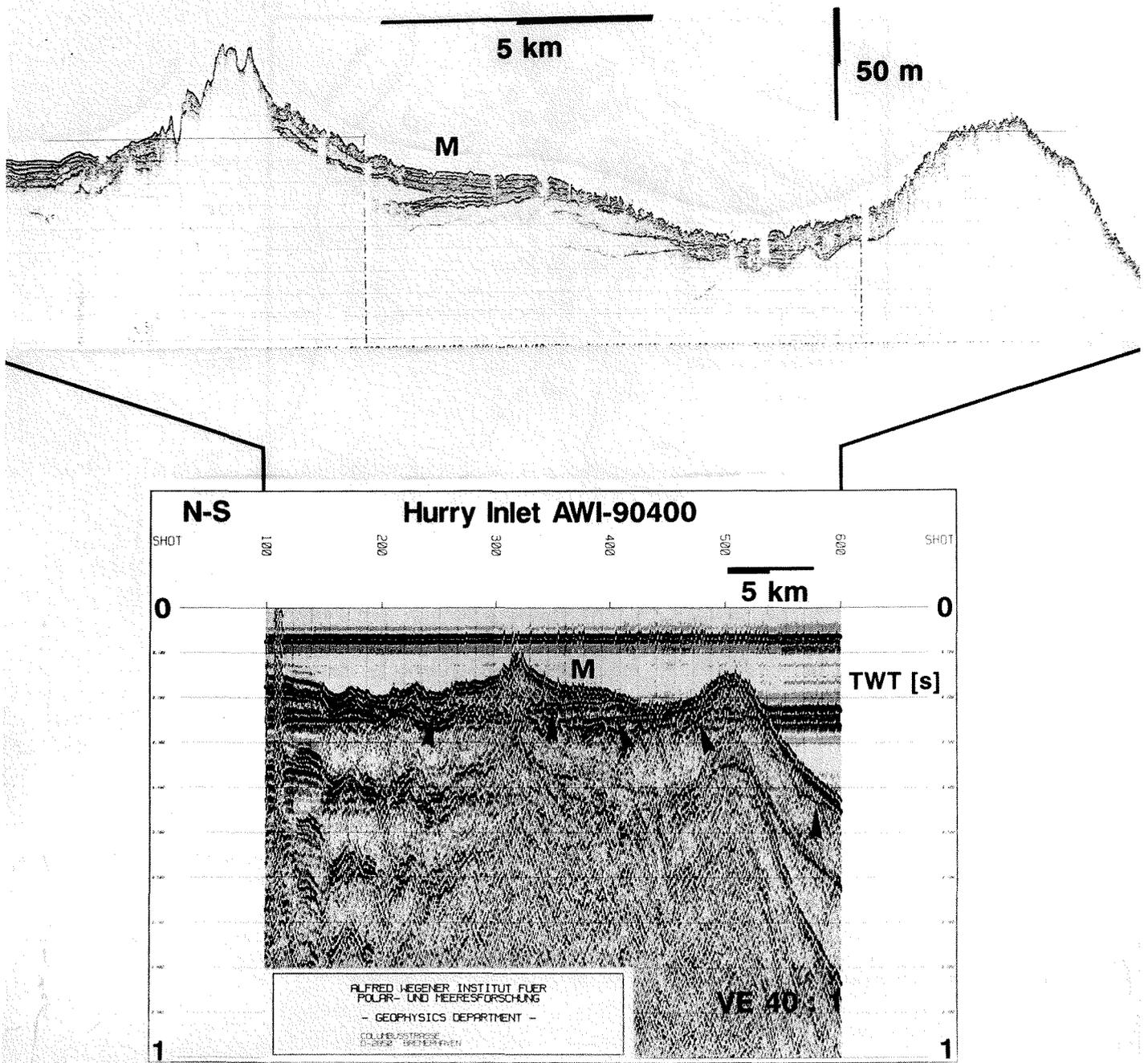
**Fig. 7:** Moraine structure (M) on line AWI-90400 in the Hurry Inlet. Parasound recording on top of seismic data. The base of the moraine can be clearly identified (Parasound and two left arrows in seismic record). The form of the structure suggests ice movements as well from the north as from the south.
