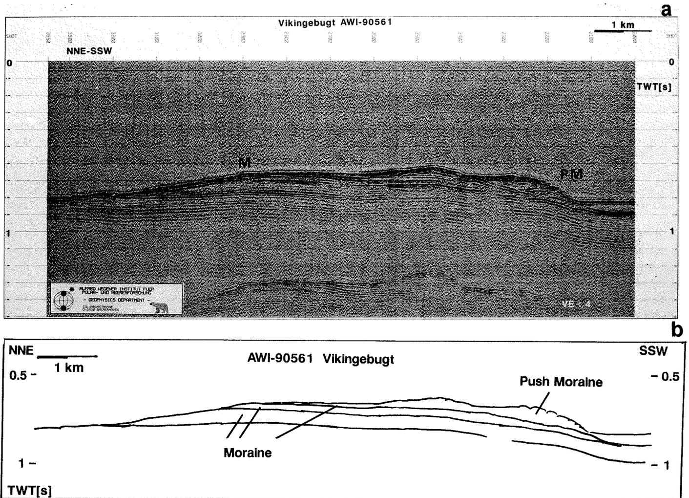
Fig. 6: a) Northern part of line AWI-90561. The mound is built up by a number of lenticular structures which are interpreted to represent moraines (M, PM). The push moraine (PM) probably documents the last ice advance. b) Linedrawing of line AWI-90561 (northern part). One can clearly see the moraines which were at least partly overridden during the different ice advances.
