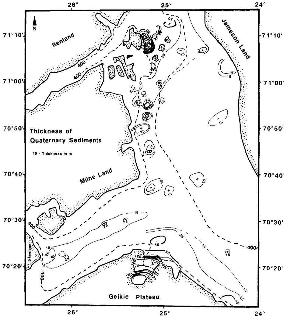
**Fig. 8:** Distribution map of Quaternary sediments. Sediments thicker than 15 m have been mapped (minimum vertical resolution of seismic data). Parasound data show that in most areas the cover is thinner than 5 m (DOWDESWELL et al. 1991). The dashed line represents the 400 m depth contour and shows that the thicker assemblages are restricted to the deeper parts of the sound.
