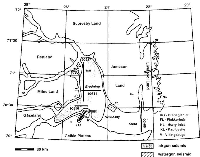
**Fig. 1:** Map of seismic investigated area in Scoresby Sund. Shaded area = airgun seismics, hatched area = watergun seismics. The thick lines show the locations of the profiles referred to in the text. During the whole experiment Parasound data were recorded.
