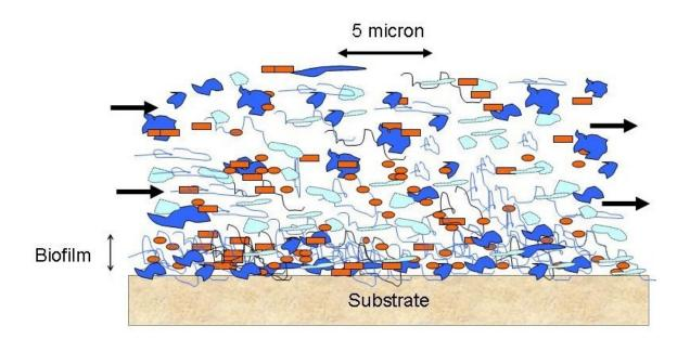
Fig 2. Schematic diagram of TEP involvement in biofilm development on a surface.
