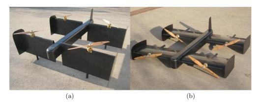
Figure 3.24: The prototype of SUAVI in vertical (a) and horizontal (b) flight modes
