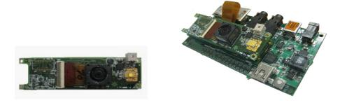
Figure 4.17: The camera solution for Gumstix
