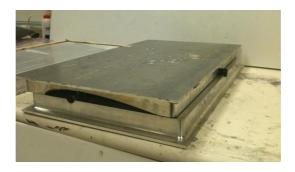
Figure 3.22: Joining two pairs of a wing between molds
