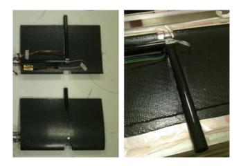
Figure 2.7: The spars and the landing gears inside the wings
