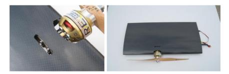
Figure 3.15: The finished wing with motor and motor driver
