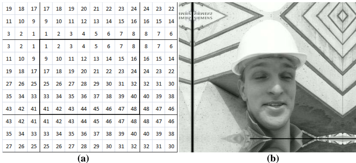
Figure 3.2: Resizing of Frames (a) 8x6 frame with resize amount = 3 (b) First frame of ForemanCIF sequence with resize amount = 32
