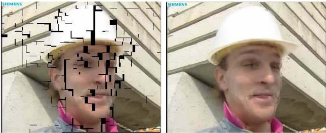
Figure 2.9: (a) Hole and Overlapping Regions (b) Frame Generated by Bilateral ME
