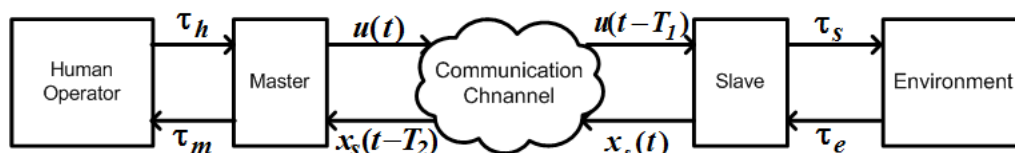
Figure 3.1: Sharing control input and position signals in observer based teleoperation systems
