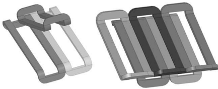
Figure 10. Balanced winding pattern implemented as final design.
