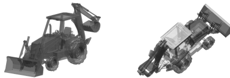
Fig. 8. Backhoe model used in Xpatch scattering predictions. The view to the right corresponds approximately to the view in the images in our experiments.
