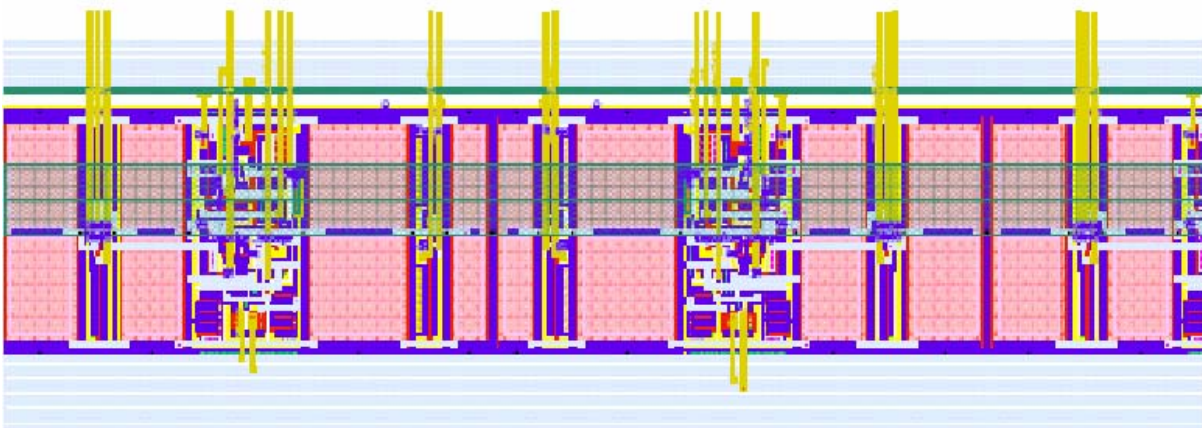
Figure 3.24: Part of layout of a channel, input capacitor sets are repeated with totally 26 in one channel, total size 56\mu\text{m} \times 2.810\text{mm} including the routing and current sources ( 400\mu\text{m} ). Channel height is dictated by pixel size.
