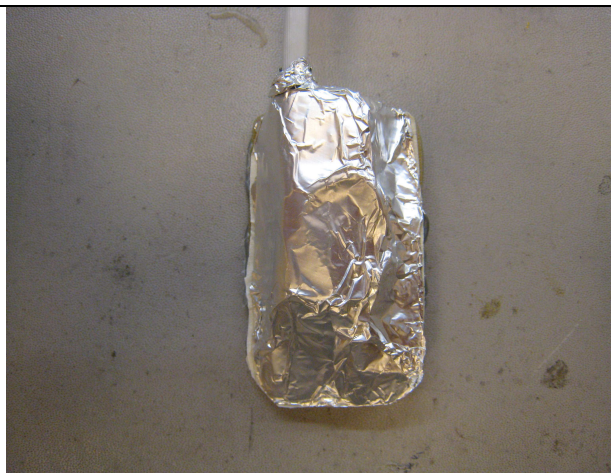
Figure 3-7 Shielding with Aluminum foil
