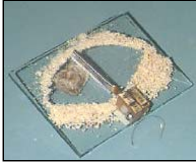
Figure 2.11 Demonstration of IPMC wipers used by NASA/JPL[42].
