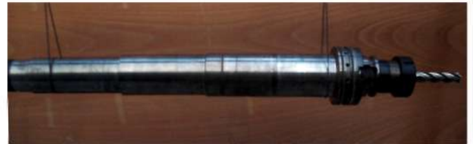
Fig. 6. Spindle-holder-tool suspended assembly for free-free measurements.
