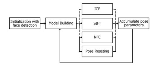
Figure 5.1: Block diagram of the tracker system
