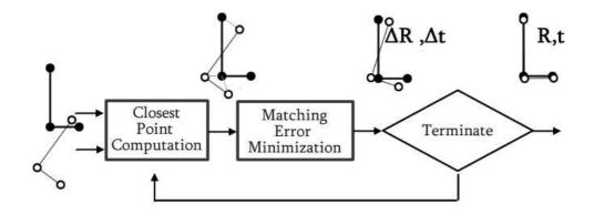
Figure 3.4: Block Diagram of ICP Algorithm
