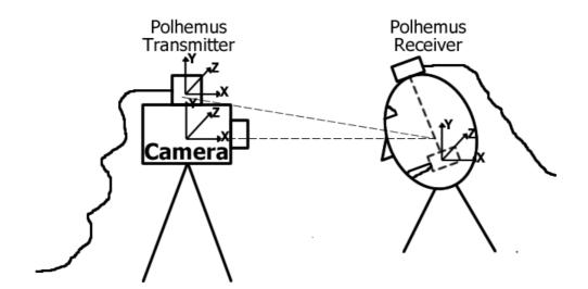
Figure 5.6: Camera and magnetic tracker coordinate systems
