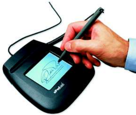
Figure 2.5: Interlink Electronics ePad-ink pressure sensitive tablet with visual feedback.
