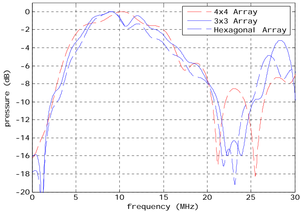
Figure 3.24 : Average pressure over the surface of arrays obtained by using ANSYS
