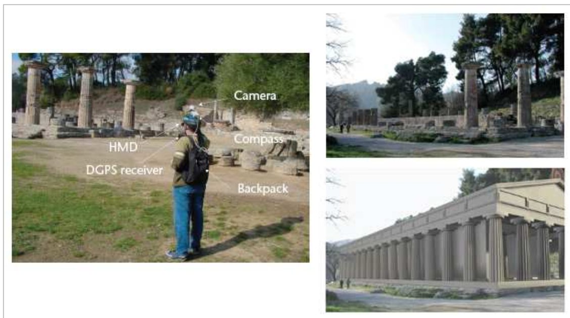
Figure 2.1 ArcheoGuide . The system setup (left), ruins of the temple (top right), augmented temple with rendered model on top of live video (bottom right) [39]
