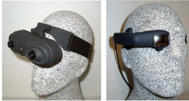
Figure 2.15 Video-see-through HMD supporting 800x600 resolution and 40° FOV diagonally (left), monocular optical-see-through HMD prototype supporting 800x600 resolution and 32° FOV diagonally (right) [38]
