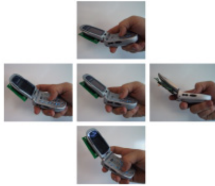
Figure 2.8 Novel interaction technique for entering text input into a mobile phone, TiltText [43]
