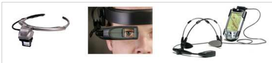
Figure 2.16 Shimadzu's Data Glass 2/A (left) [37], Liteye's Liteye-500 (middle) [28], Icuiti's M-920CF with a PDA setup (right) [19].
