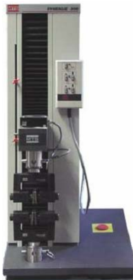
Figure 8 MTS Synergie 200 tensile testing apparatus with pneumatic rubber clamps (In courtesy of Rotopak-Alcan Packaging)
