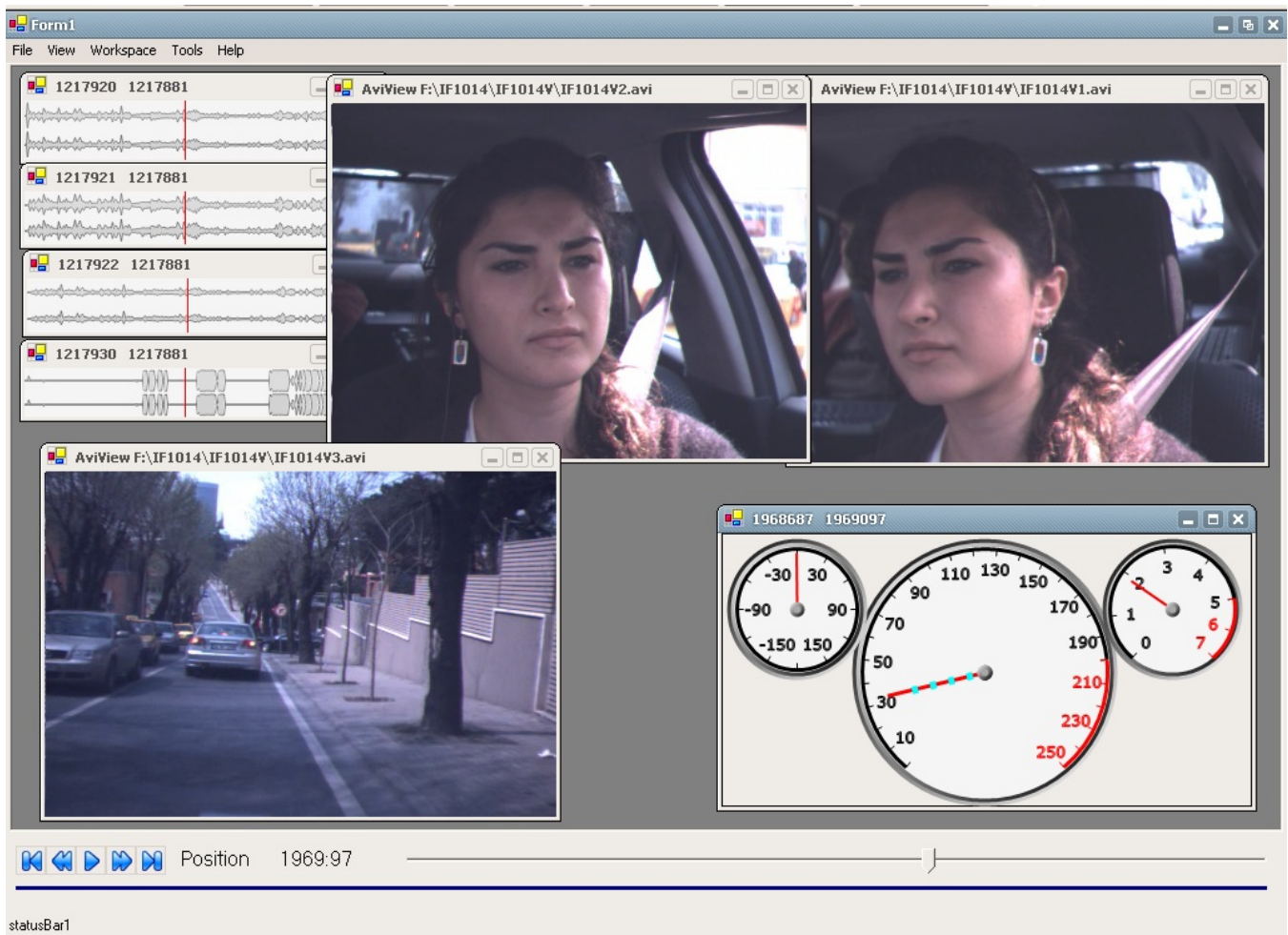
Figure 5. The browser synopsis of the Multi-channel Multimedia Display for Driver IF1014. Three video feeds and 4 audio waveforms together with steering wheel angle, vehicle speed, and engine rpm dials are included in this pictures. In addition four blue dots represent the individual speeds in each tire of the vehicle.
