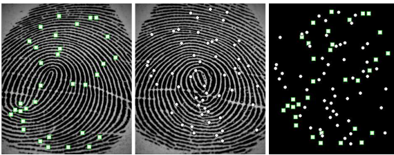
Figure 1. The combined fingerprint minutiae on the right is what is stored at the central database. The source finger of minutiae points are actually lost; they are marked here with special shapes for clarity.
