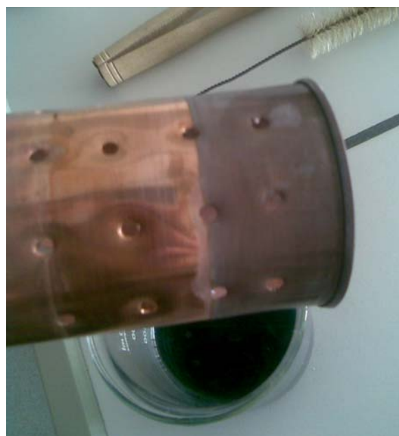
Figure 3: Shows the cathode after the experiment with copper (II) chloride.
