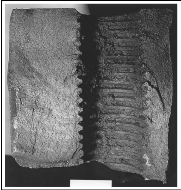
Fig. 10 Fractograph of the wheel hub fatigue failure
