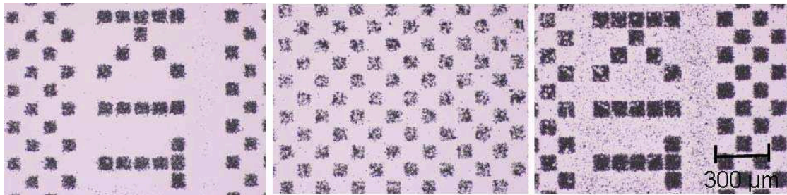
Figure 4.10: Glycine particles printed on the glass slide. The three figures are parallel on the slide. Left, middle, and right figures correspond to the left, middle, and right slide area, respectively. The particles on both sides are more than the particles in the middle.
