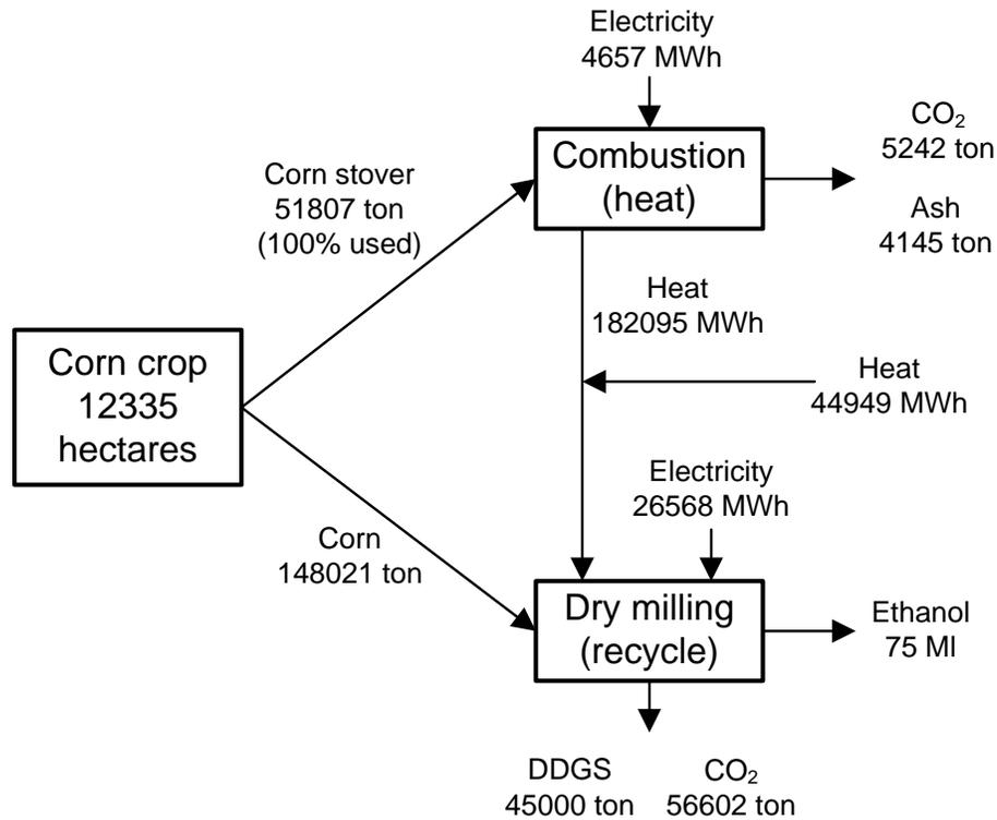
**Figure 3.8:** Overall process - Configuration 2
