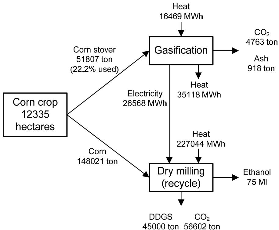
**Figure 3.14:** Overall process - Configuration 8
