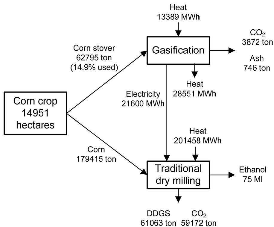
**Figure 3.13:** Overall process - Configuration 7
