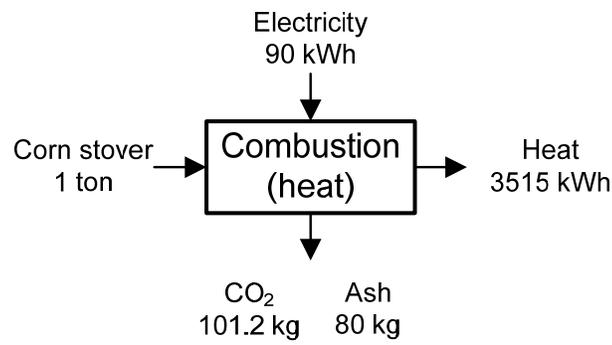
**Figure 3.4:** Model of combustion process for heat generation
