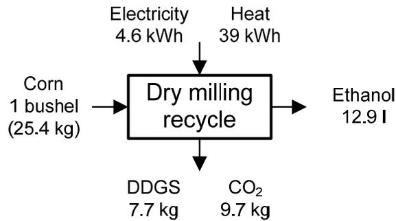
**Figure 3.2:** Model of dry milling with recycle process
