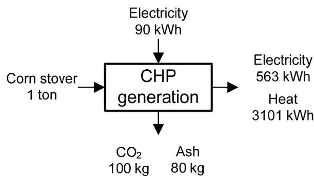
**Figure 3.5:** Model of combustion process for heat and electricity generation
