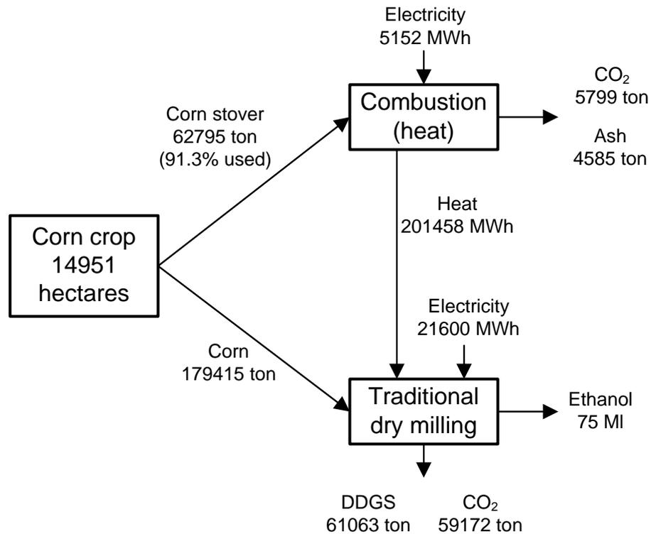
**Figure 3.7:** Overall process - Configuration 1
