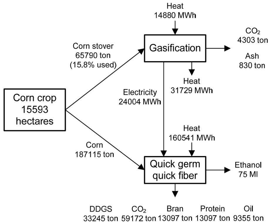
Figure 3.15: Overall process - Configuration 9
