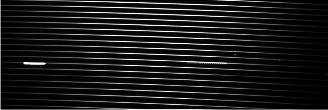
Figure 2.1: An echelle spectrum of 4 CVn taken at McDonald observatory. Every white line is one echelle order. The wavelength increases from bottom to top and from right to left, spanning a total range of 4200 Å to 4700 Å. The picket fence is the bright spot on the eighth and ninth line from the bottom. It appears twice, because the orders are overlapping. The white dots are cosmic rays.
