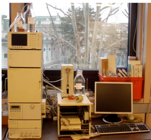
Figure 25: HPLC LC-10 AD, Shimadzu; Department of Pathophysiology and Allergy Research; Medical University of Vienna
