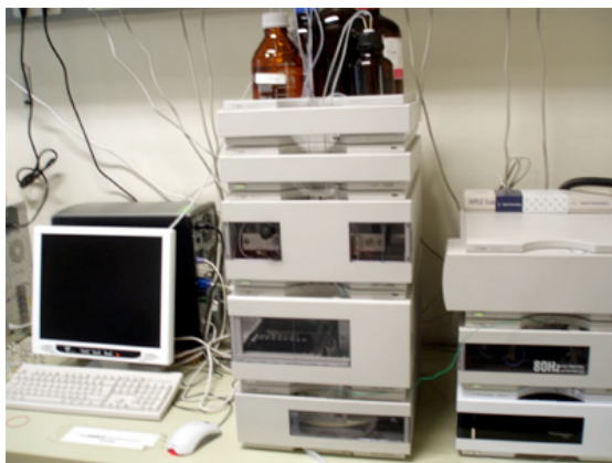
Figure 26: HPLC Agilent 1100 Series; Department of Systematic and Evolutionary Botany; Faculty Centre of Biodiversity of the University of Vienna
