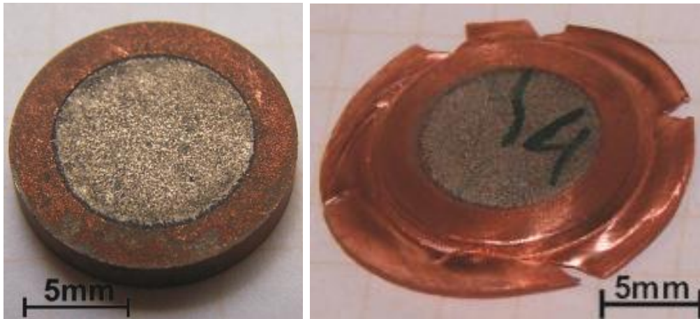
Fig. 3-8. Magnesium samples with Cu ring attached prepared for HPT experiments (on the left hand), and the same sample after HPT deformation at the right hand (mark on the sample attached for verification of the number of rotations applied).
