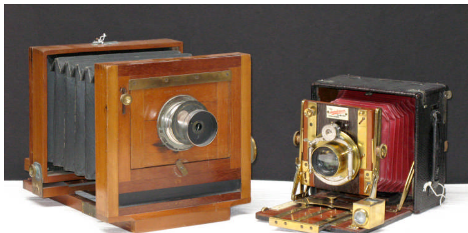
Figure 6.16: Two large format cameras showing the rapid evolution of the field type camera. On the left a circa 1885 Scovill 5x7 Elite camera with original single element landscape lens. On the right a circa 1905 Sanderson quarter plate Junior camera with original Cooke 7.87 inch lens; Frederick Evans used a similar Sanderson camera (collection of the author).
