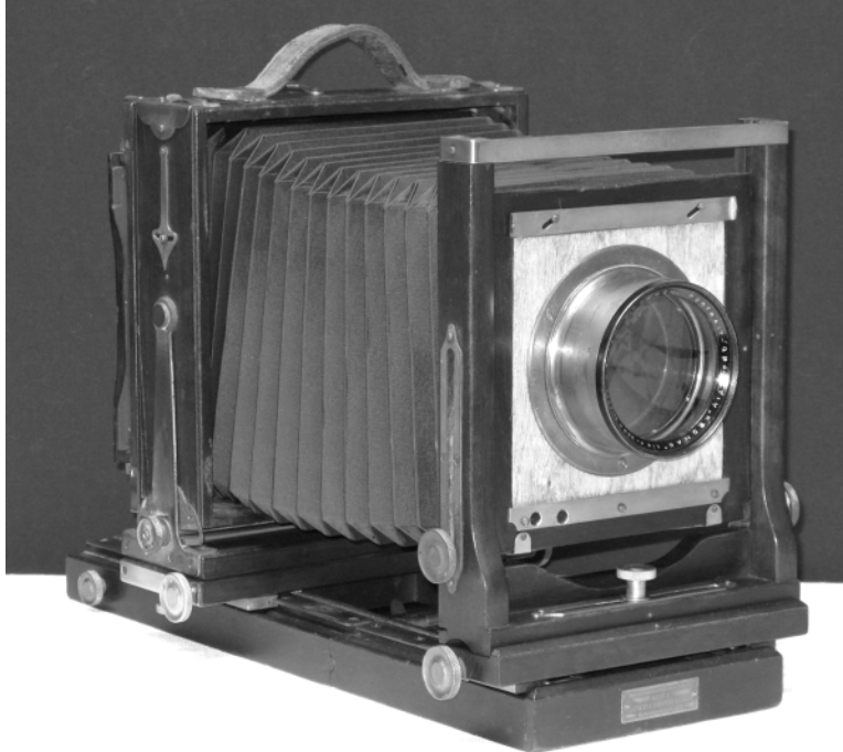
Figure 6.20: Agfa-Ansco 5x7 view camera circa 1925 with a contemporaneous Portrait-Objectiv Kronar f/4 350mm soft focus lens made by Simon, Dresden. Moderately compact when collapsed, possessing limited movements, 23 inch bellows and 5¼ inch square lens board, this type of camera was ideal for the pictorialist who required a versatile camera to also be portable (collection of the author).
