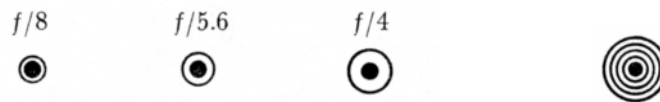
Core image and halo of the Verito , greatly exaggerated (with kind permission, Albert Starkweather “Notes on the Verito Lens”) 92
