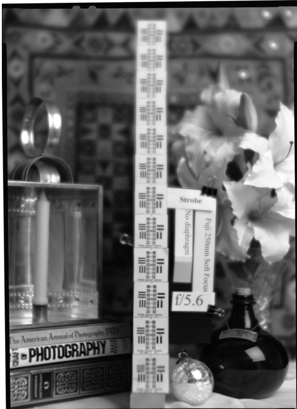
Figure 5.10: Fujinon SF 250 mm f /5.6 ca. 1985, on a 5x7 negative reproduced 100% size. Compared to the Gundlach lens, it has much less flare and is somewhat firmer, both characteristics of post-1970 soft focus lenses. Like most post-1970 lenses, it lacks the ‘sparkle’ of the pre-1930 lenses. Photograph by the author.
