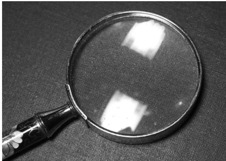
Figure 5.7: Two reflections of the same light source on an uncoated magnifying glass lens. One reflection is from the front surface, the other from the rear surface of the glass. This would produce substantial flare if the lens was used to project an image under these lighting conditions (photograph by the author).
