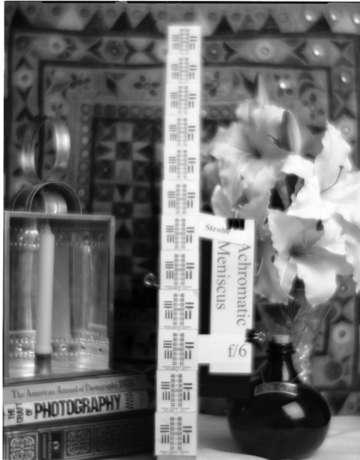
Figure 5.9: Gundlach Achromatic Meniscus 6 inch f/6 ca. 1920 on a 4x5 negative reproduced 100% size, a relatively high flare soft focus lens and a very agreeable softness. Photograph by the author.
