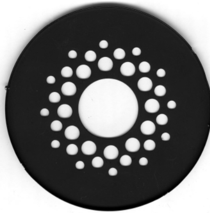
Figure 6.9: Perforated diaphragm from an Imagon lens, 420 mm focal length, manufactured circa 1934. In 1935 the circles of perforations were reduced from three as seen here to two which undoubtedly changed the degree of diffusion by reducing the amount of marginal rays 37 (collection of the author).
