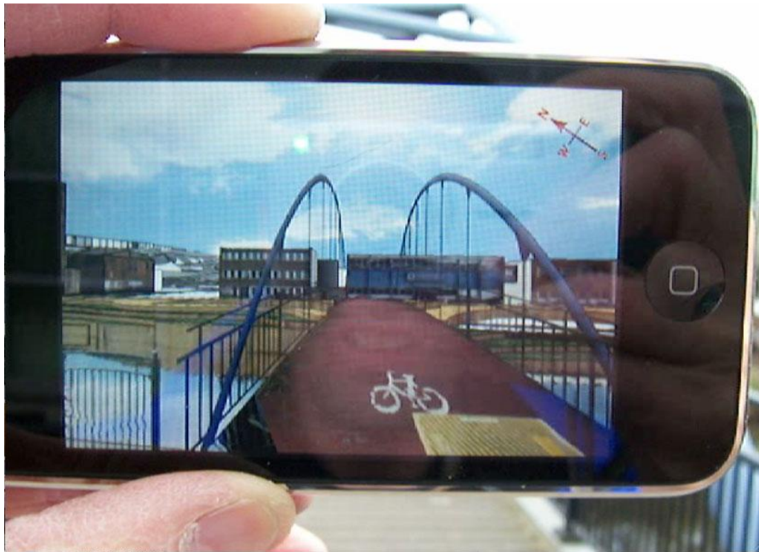
Figure 1 Mobile phone augmented reality. For spatial reference, notice the railing in the visualization and in the real world. In the future, will we all be using our mobile phones to look at planning proposals on site?
