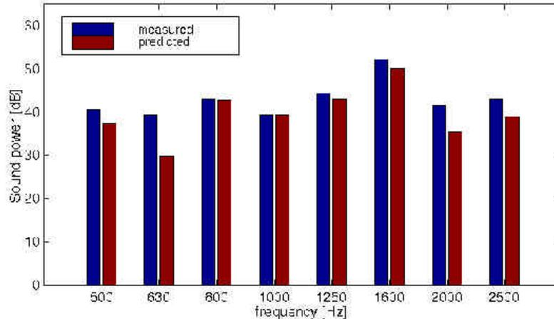
Figure 4: Measured and predicted radiated sound power for the running induction motor.
