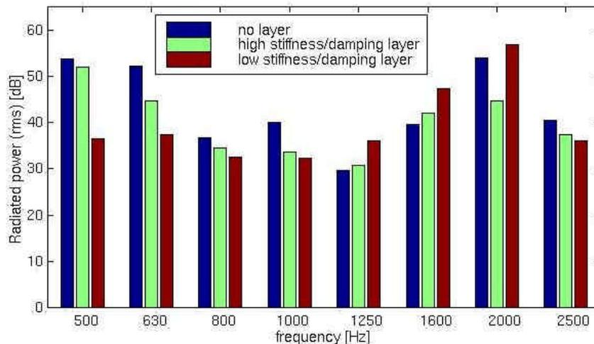
Figure 5: Radiated acoustic power level of a motor with and without viscoelastic supports.
