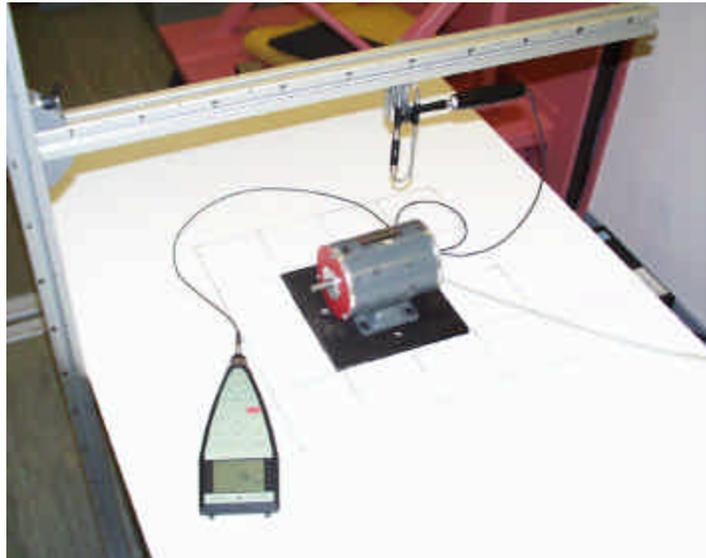
Figure 3: Setup for acoustic intensity measurements of the electric motor.
