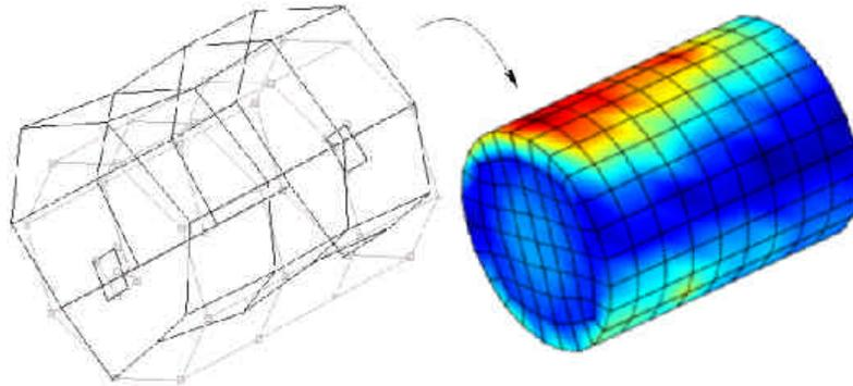
Figure 2: Measured normal velocity projected on a BEM model for a specific frequency.
