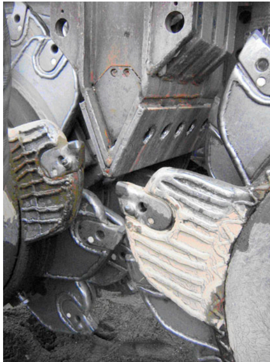
Figure 4. The trench-cutter Bauer BC 30 used to realise the Turin underground railway link: details of the rotating excavation head.
