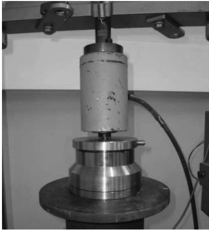
(A) DRAINED CONSOLIDATION OF SPECIMEN #1
