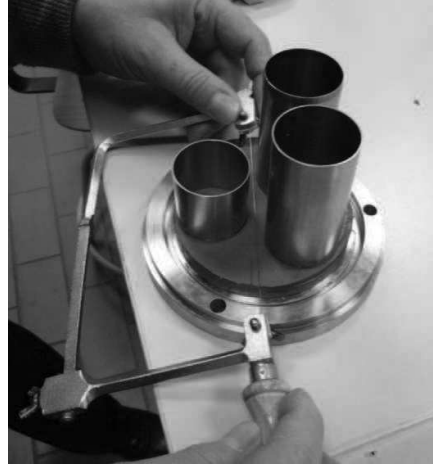
(B) SPECIMEN #1 CROP WITH 38.1 mm MOLD OBTAINING SPECIMENS 1A, 1B AND 1C
