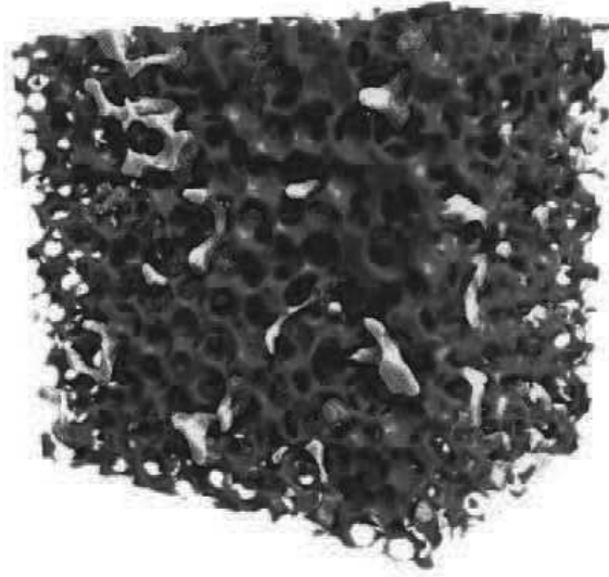
Figure 4.1 – Schematic representation of the residual condition of the wetting phase in a porous medium.
