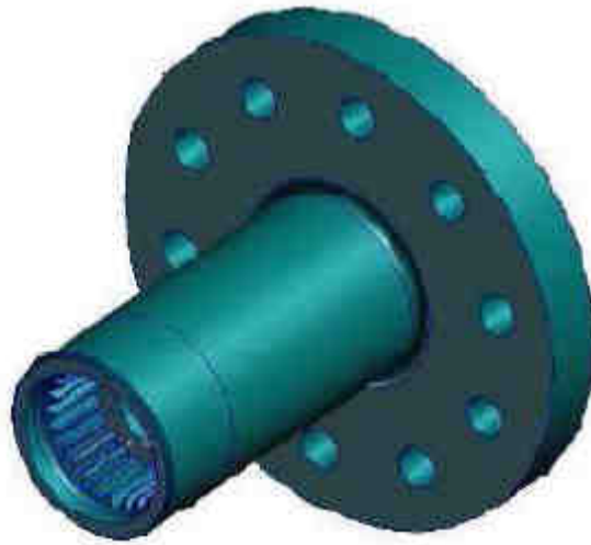
Figure 3.14: External spline coupling (hub)
