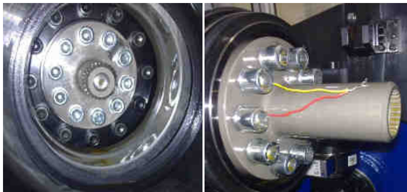
Figure 6.1: Test Article mounted on the test bench; to the left there is the shaft and to the right there is the hub
