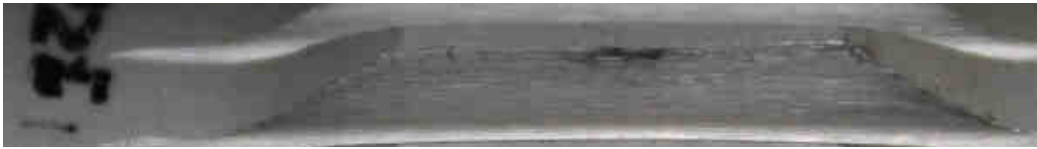
Figure 6.2: Image of the 19th tooth of the specimen MB1 before test
