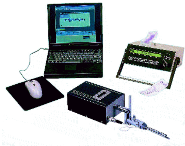
Figure 5.21: surface roughness tester RT-70
